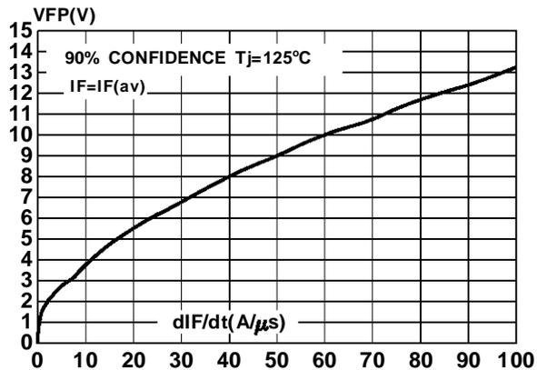
Fig 15 : Forward recovery time versus  $dI_F/dt$
