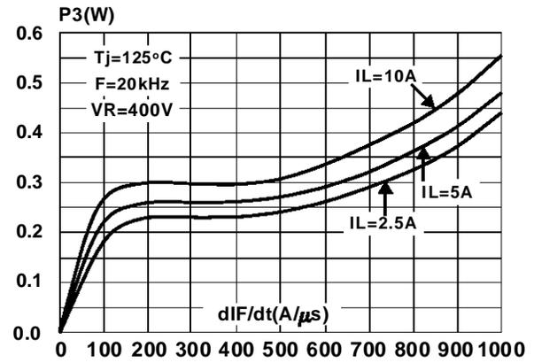
Fig 7 : Switching ON losses versus  $dIF/dt$
