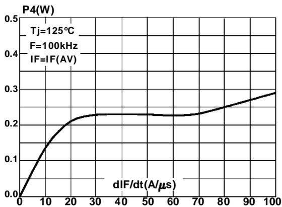
Fig 8 : Switching losses in transistor due to the diode
