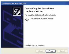
7. When the **Finish** button is clicked in step 6, the installation of the USB Serial Port driver will be automatically started.
