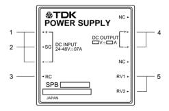
Between RC and input (–): Turned off at low level (0 to 0.4V) or in short circuit
