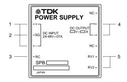
Between RC and input (–): Turned off at low level (0 to 0.4V) or in short circuit.
