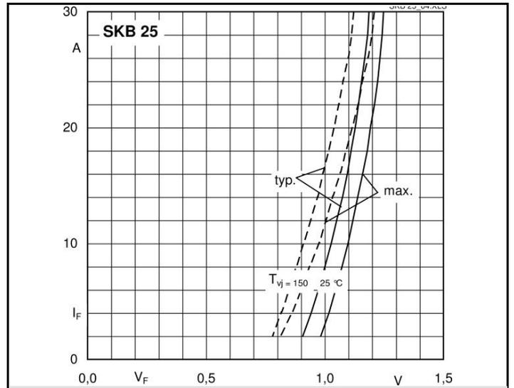
Fig. 9 Forward characteristics of a diode arm
