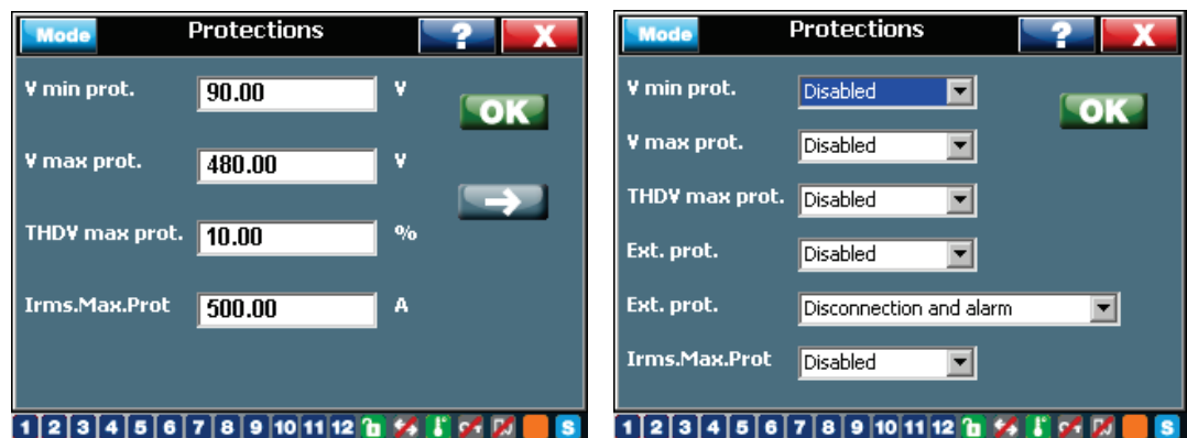
Figure 40: RVT protection settings
