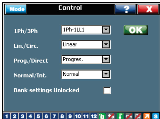
Figure 34: RVT bank settings protection: not protected
