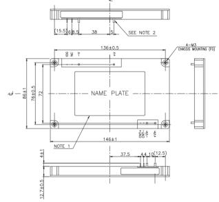
Note 1: Model name, Input voltage range, Nominal output voltage, Maximum output current and country of manufacture are shown here.
