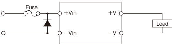
Fig.1-5 Protection for Reversed Input Connection
