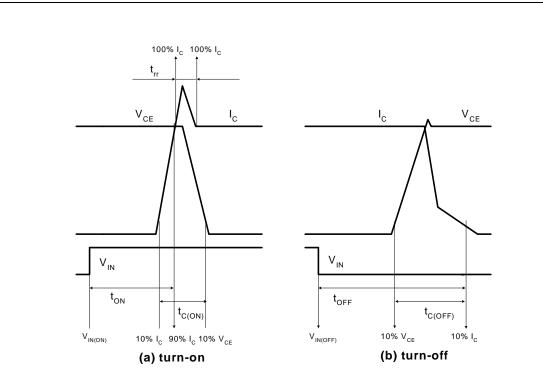
Figure 4. Switching Time Definition
