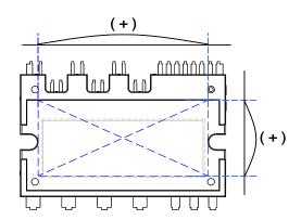
Figure 7. Flatness Measurement Position
