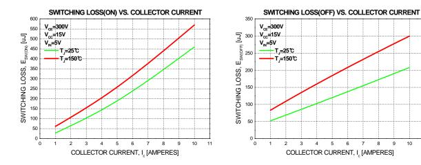
Figure 5. Switching Loss Characteristics
