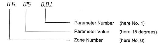
In this example, the high temperature alarm for zone no. 6 is activated at 15 degrees above setpoint.
