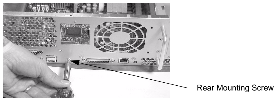
Figure 3-54. Removing the System Boards Rear Mounting Screw
