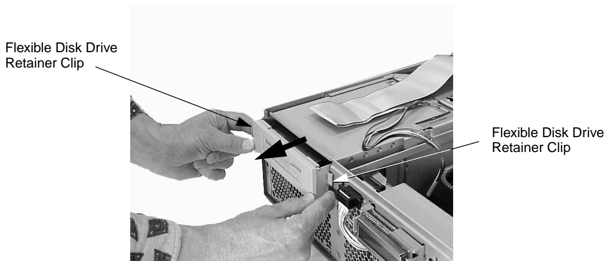
Figure G-2 Remove the Flexible Disk Drive and Flexible Disk Drive Bay
