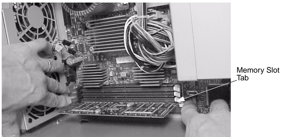
Figure 3-3. Pressing Down on the Memory Slot Tabs
