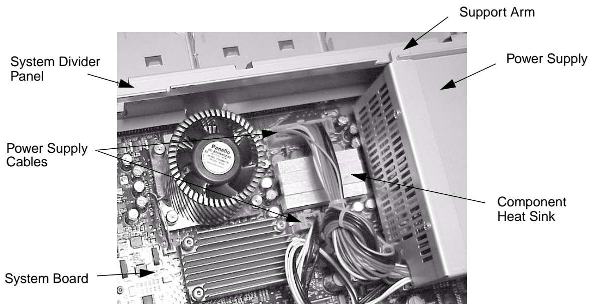
Figure 3-47. Disconnect the Power Supply Cables
