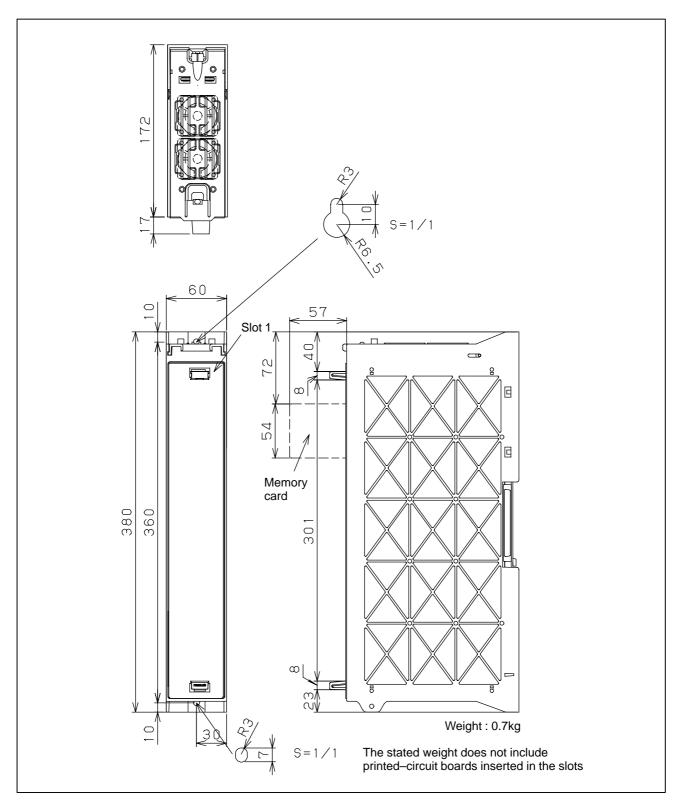
Fig.U1 Series 0*i* Mate–B basic unit (1–slot) Specification No. : A02B–0301–B801
