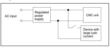
For a circuit configuration in example 2, connect another regulated power supply to be specifically used for the device with remarkable load fluctuations so that the CNC and other units are not affected.
