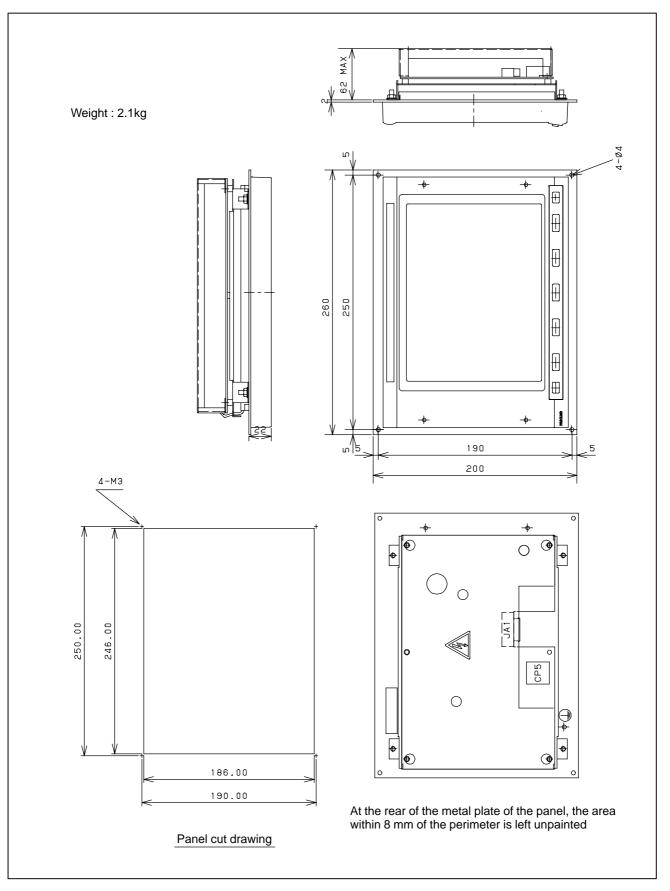
Fig.U6 8.4" TFT color LCD unit Specification No. : A02B–0299–C080
