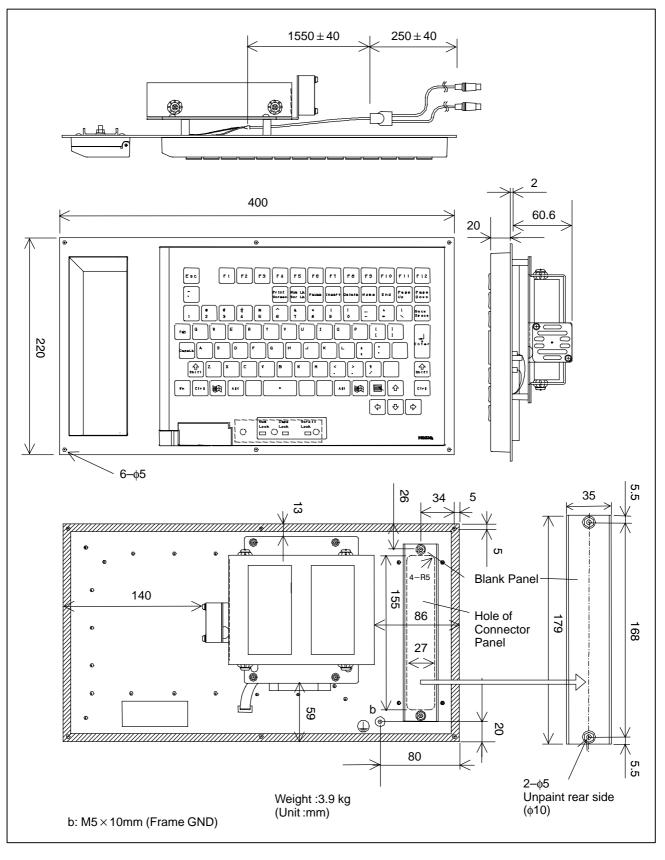
Fig.U12 (c) FA Full Keyboard 15.0" LCD Type Specification N. : A08B-0082-C150#JC, A08B-0082-C150#EC
