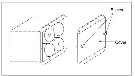
(4) After installing the new batteries, replace the cover.
