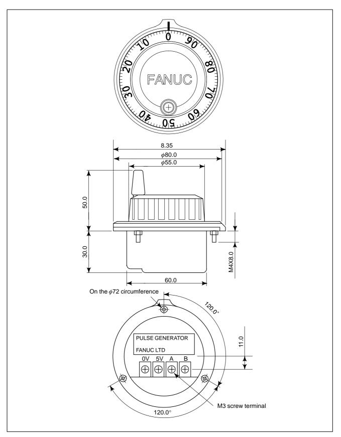
Fig.U18 Manual pulse generator Specification No. : A860–0202–T001
