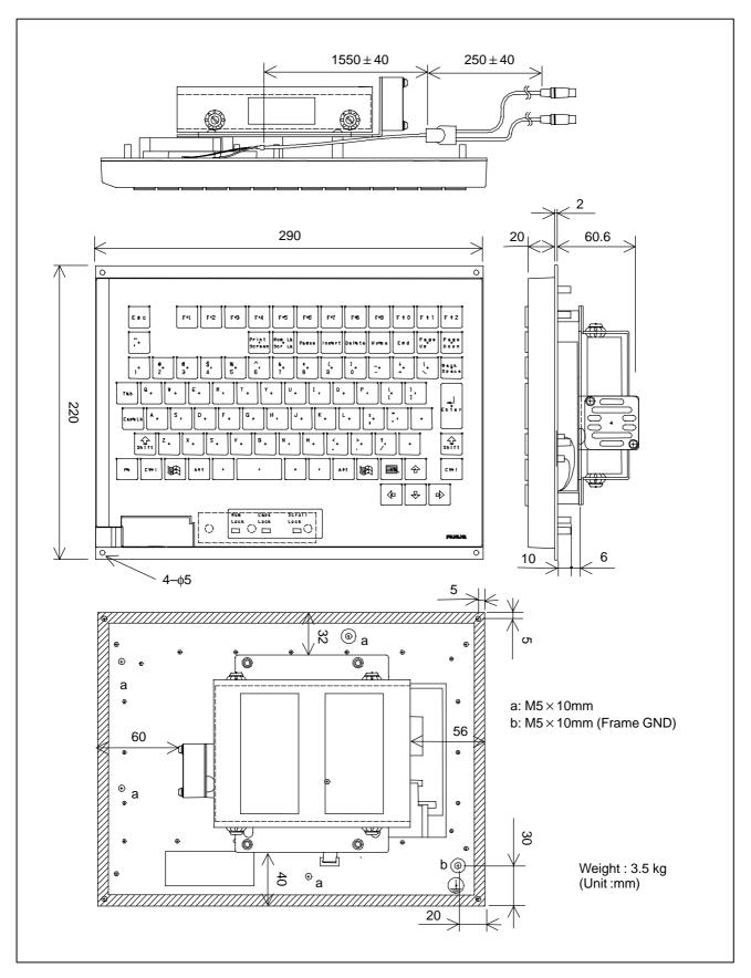
Fig.U12 (a) FA Full Keyboard 10.4" LCD Type Specification No. : A02B-0236-C131#JC,A02B-0236-C131#EC
