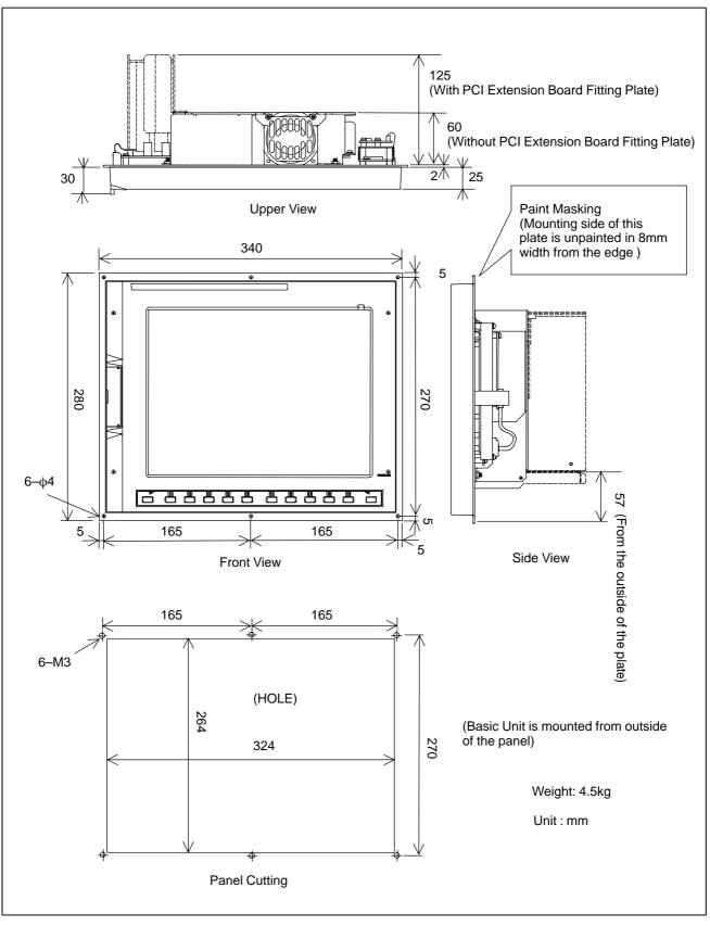
Fig.U10 (b) 12.1" TFT color LCD of CNC display unit with PC functions
