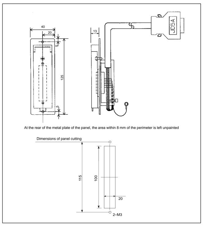
Fig.U24 Punch panel (narrow width type) Specification No. : A02B–0120–C191 (Cable length : 1m) A02B–0120–C192 (Cable length : 2m) A02B–0120–C193 (Cable length : 5m)
