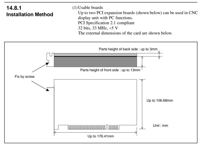
(2) Method of mounting PCI extension board
