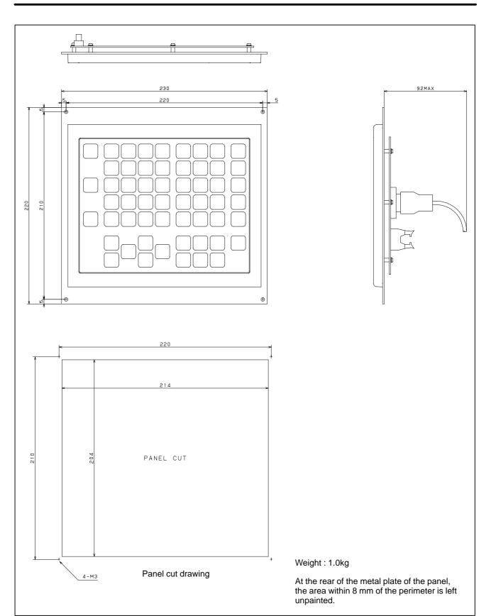
Fig.U30 Separate type MDI unit (full–key) Specification No. : A02B–0279–C121#MA, #TA (English display MDI) A02B–0279–C121#MAS, #TAS (Symbol display MDI) A02B–0279–C121#MB, #TB (English and symbol display MDI)
