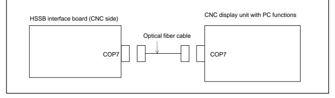
1) Recommended cables (optical fiber cables)
