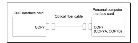
Usable Optical Fiber Cable (The FSSB optical fiber cable to be used outside of the cabinet.)
