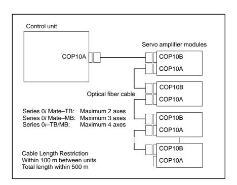
The connection between the CNC control unit and the servo amplifiers should use only one optical fiber cable, regardless of the number of controlled axes. See APPENDIX D for details on the optical fiber cable.
