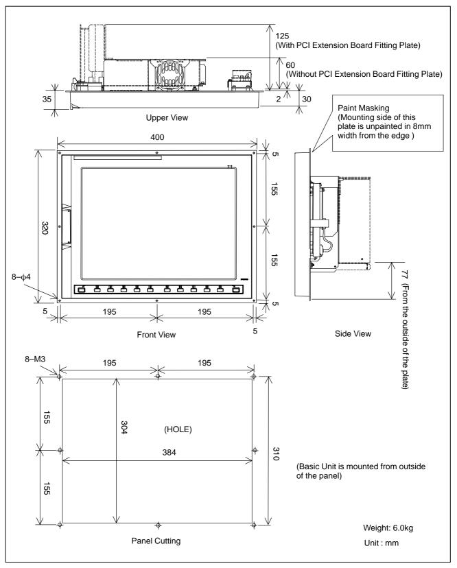
Fig.U10 (c) 15.0" TFT color LCD of CNC display unit with PC functions
