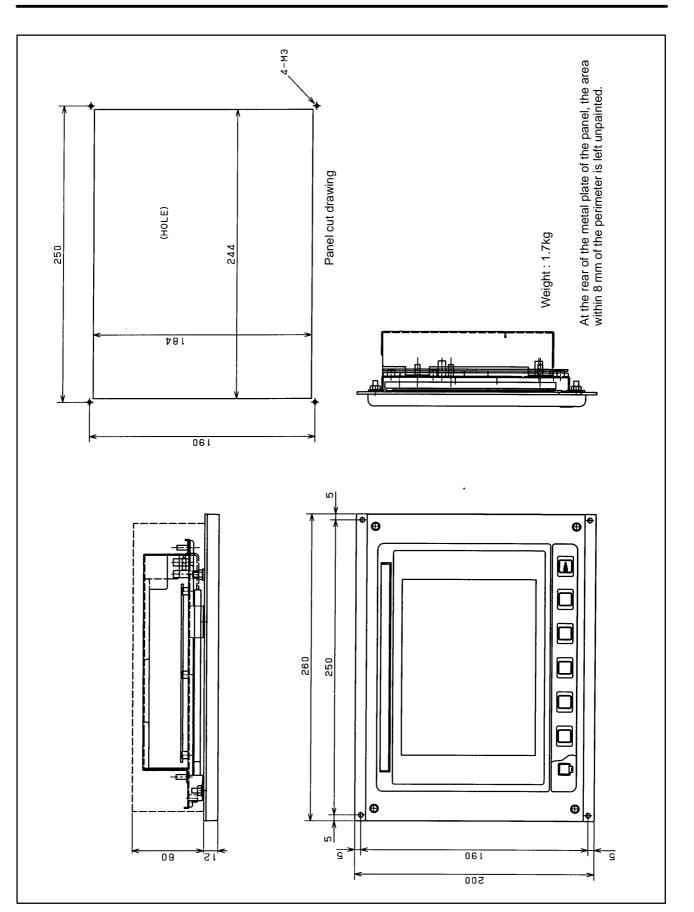
Fig.U28 7.2" STN monochrome LCD unit Specification No. : A02B–0299–C070, C075
