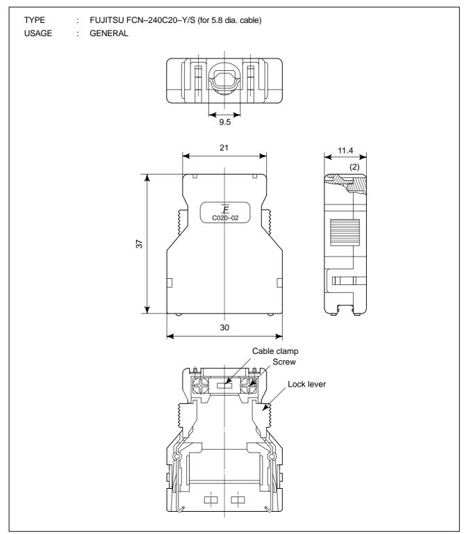
Fig.C2 (c) Connector case (FUJITSU FCN type)
