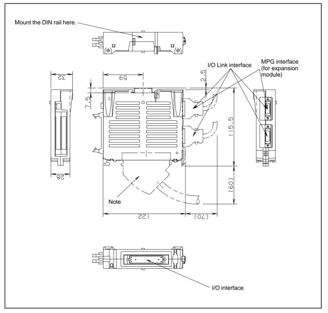
When mounting a DIN rail (external module view and mounting diagram)
