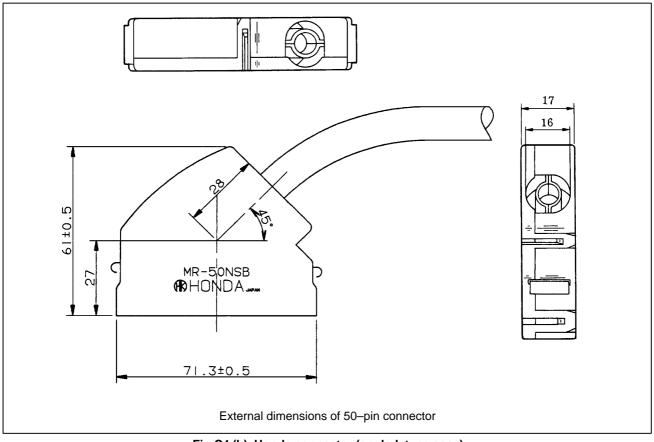
Fig.C4 (b) Honda connector (angled-type case)
