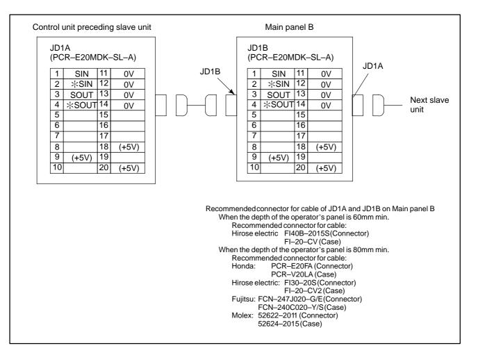
+5V terminals are for an optical I/O Link adapter. They are not necessary when connecting with a metal cable.
