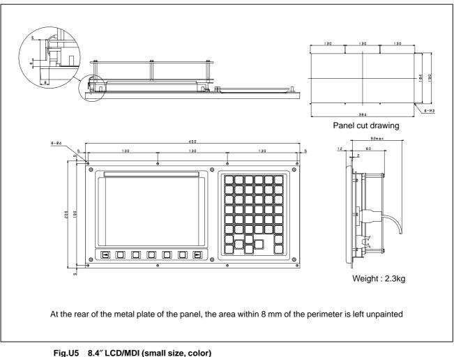
Fig.U5 8.4″ LCD/MDI (small size, color) Specification No. : A02B–0299–C081#M, #T (English display MDI) A02B–0299–C081#MS, #TS (Symbol display MDI) A02B–0299–C081#MB, #TB (English and symbol display MDI)
