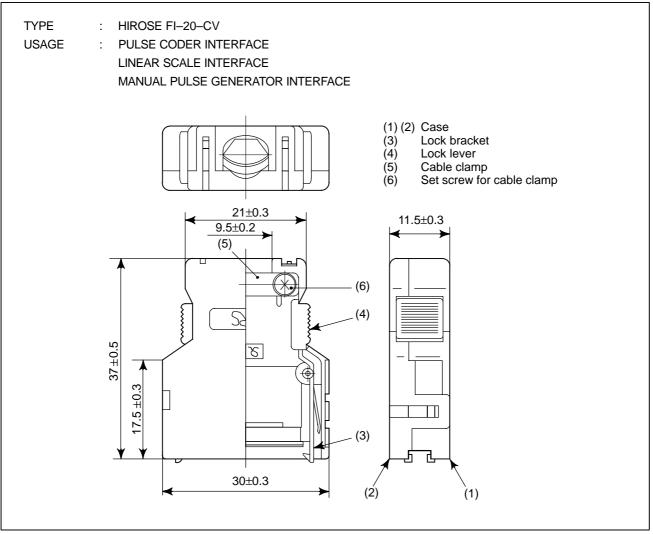
Fig.C2 (b) Connector case (HIROSE FI type)
