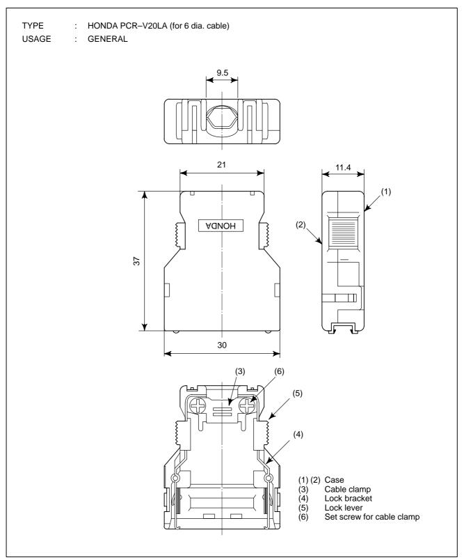
Fig.C2 (a) Connector case (HONDA PCR type)
