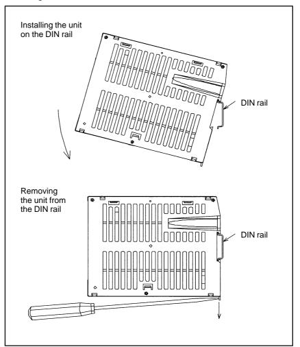
Installing the unit on the DIN rail
