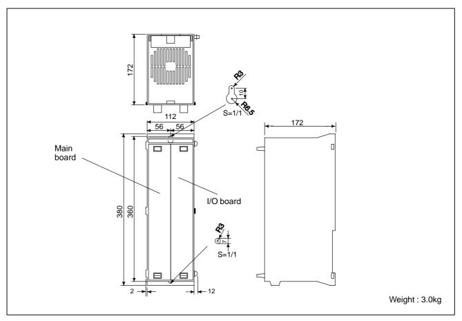
Fig.U2 Series 0*i*–B basic unit (2–slot) Specification No. : A02B–0299–B802
