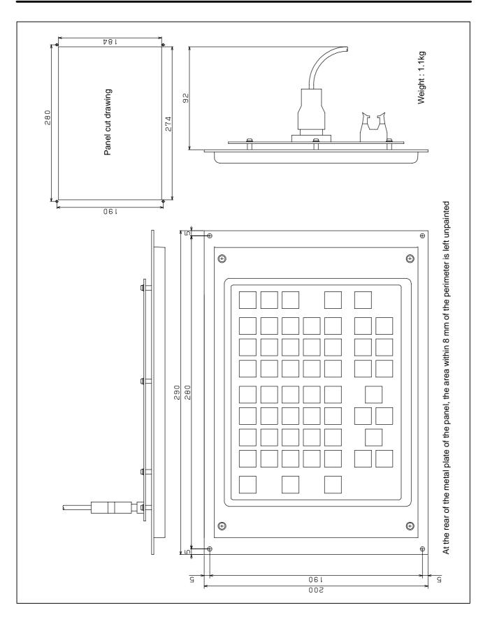
Fig.U9 Stand–alone type MDI unit (full–key) Specification No. : A02B–0279–C122#MA, #TA (English display MDI) A02B–0279–C122#MAS, #TAS (Symbol display MDI) A02B–0279–C122#MB, #TB (English and symbol display MDI)
