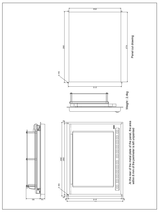
Fig.U7 10.4" TFT color LCD unit Specification No. : A02B–0299–C060
