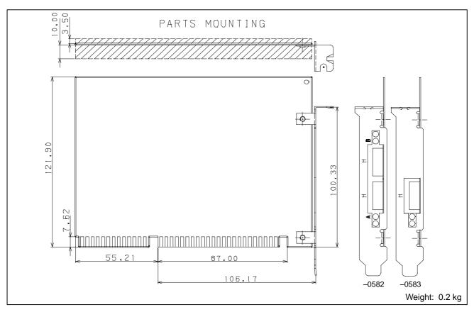
Fig.U16 (a) High-speed serial bus interface board type 2 (PC) (ISA bus version) Specification No. : A20B-8001-0583 (1 CH) A20B-8001-0582 (2 CH)
