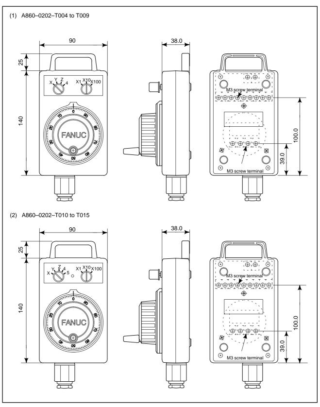
Fig.U19 Pendant type manual pulse generator Specification No. : A860–0202–T004 to T015
