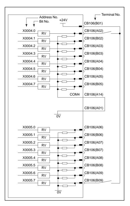
For address X0004, either a source or sink type (with a 0– or 24–V common voltage) can be selected. COM4 must be connected to either 24 or 0 V; never leave it open. From the viewpoint of safety standards, it is recommended that a sink type signal be used. The above diagram shows an example in which the signal is of sink type (with a 24–V common voltage).
