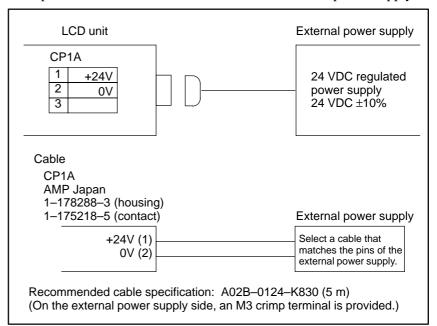
Part of the 24 VDC power input to CP1A can be taken out from CP1B by branching. CP1B should be connected as shown below. In this case, the rating of the external 24 VDC power supplied to CP1A must be the sum of the power consumed within the control unit and that supplied to external equipment via CP1B. Up to 1.4 A can be supplied to the external equipment.
