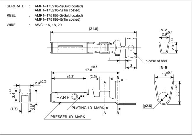
Fig.C3 (e) Contact for AMP connector
