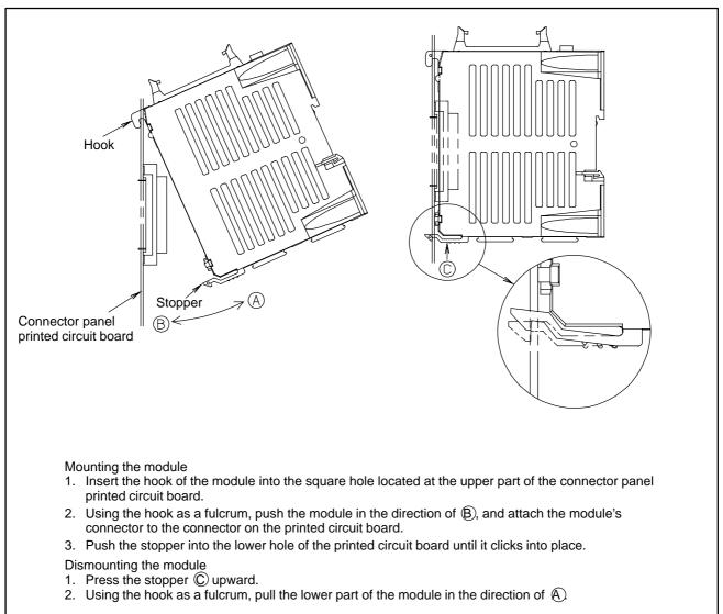
When connecting a connector panel printed circuit board directly (mounting and dismounting a module)
