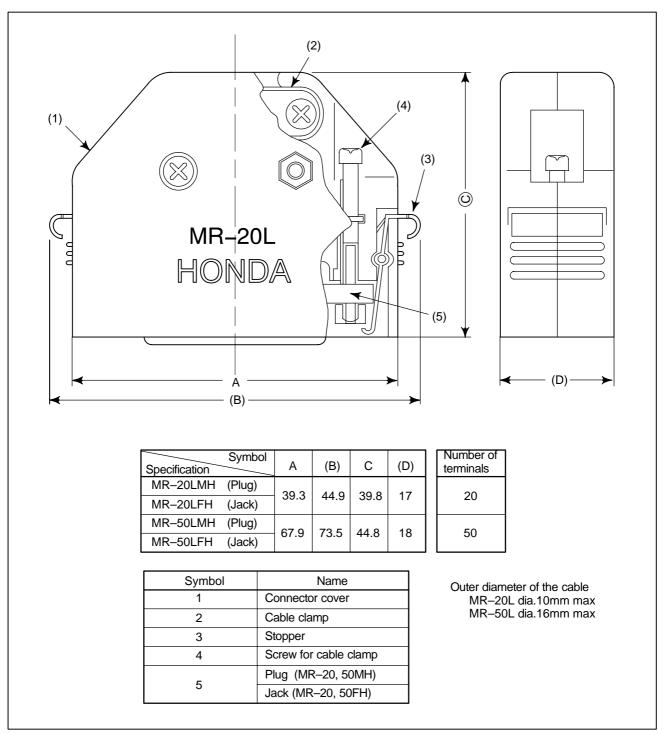
Fig.C4 (a) HONDA connector (case)
