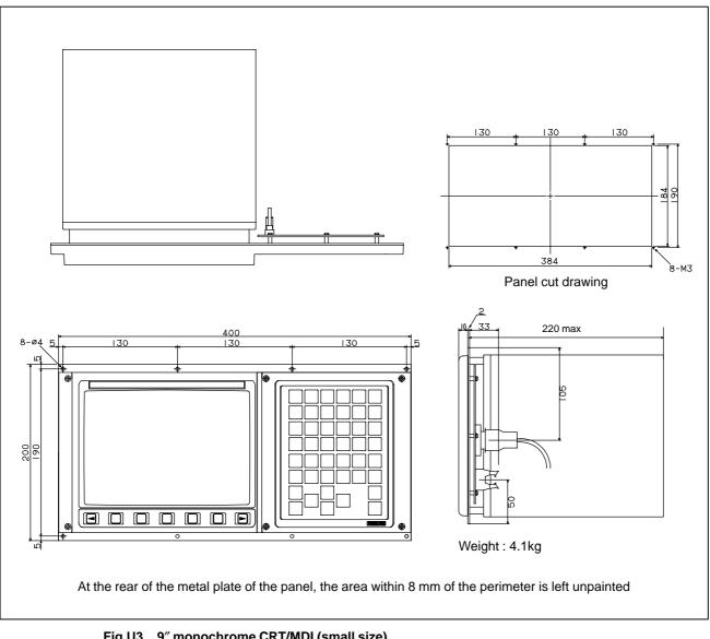
Fig.U3 9<sup>″</sup> monochrome CRT/MDI (small size) Specification No. : A02B–0299–C041#M, #T (English display MDI) A02B–0299–C041#MS, #TS (Symbol display MDI) A02B–0299–C041#MB, #TB (English and symbol display MDI)
