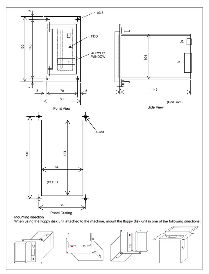
Fig.U15 Floppy disk unit Specification No. : A20B–0207–C008
