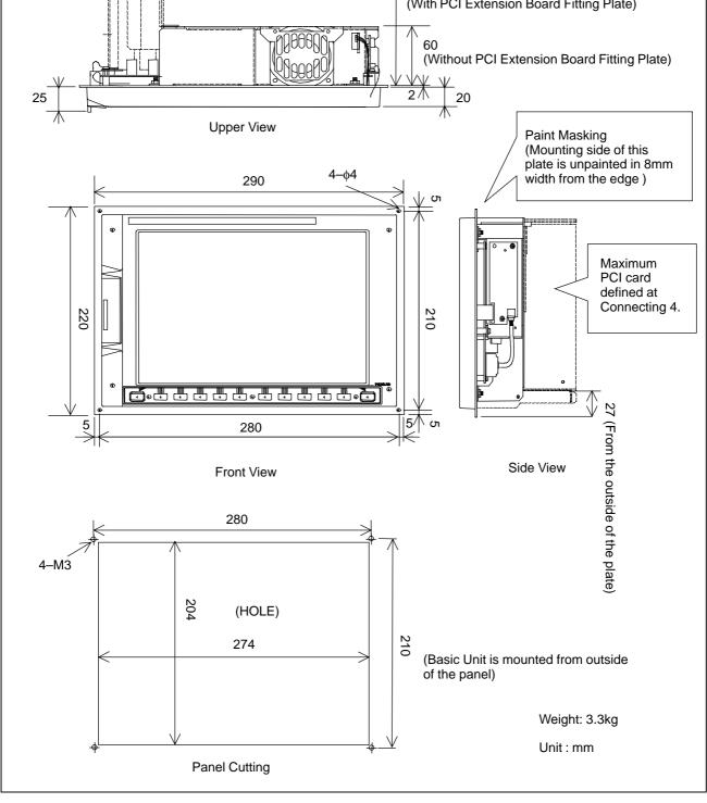
Fig.U10 (a) 10.4" TFT color LCD of CNC display unit with PC functions
