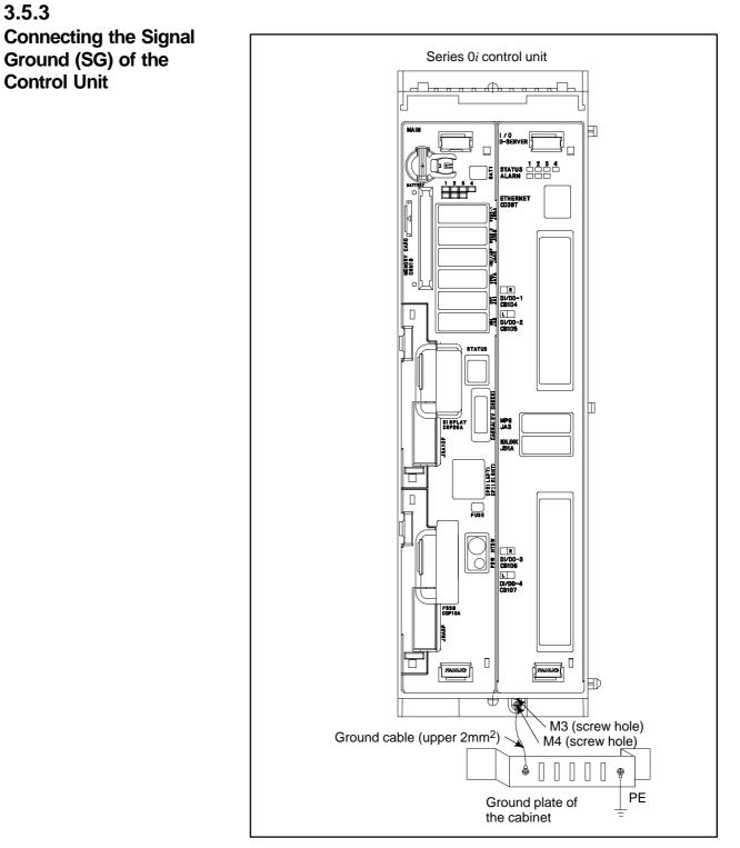
Connect the 0 V line of the electronic circuit in the control unit with the ground plate of the cabinet via the signal ground (SG) terminal. The SG terminal is located below the main board of the control unit.
