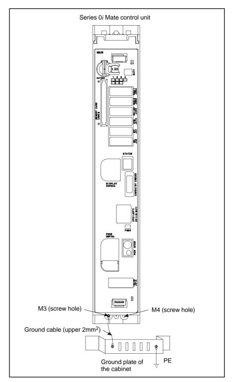
Connect the 0 V line of the electronic circuit in the control unit with the ground plate of the cabinet via the signal ground (SG) terminal. The SG terminal is located below the main board of the control unit.
