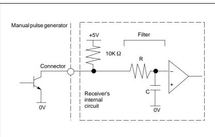
The circuit to receive the signal of the manual pulse generator is as shown in the figure below.
