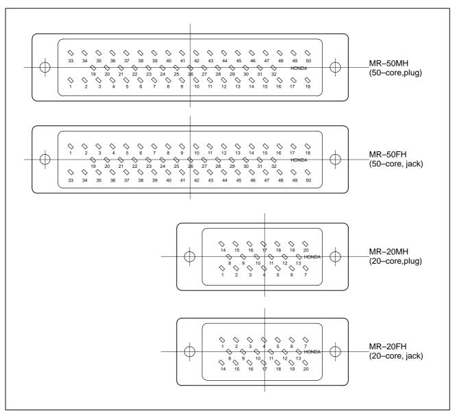
Fig.C4 (e) HONDA connector (terminal layout)
