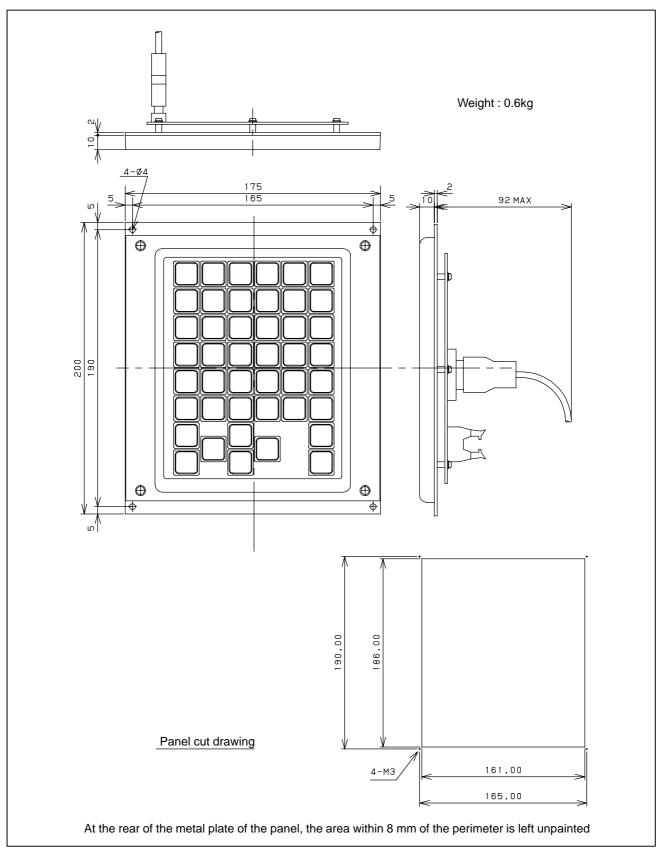
Fig.U8 Stand–alone type MDI unit (small size) Specification No. : A02B–0279–C120#MA, #TA (English display MDI) A02B–0279–C120#MAS, #TAS (Symbol display MDI) A02B–0279–C120#MB, #TB (English and symbol display MDI)
