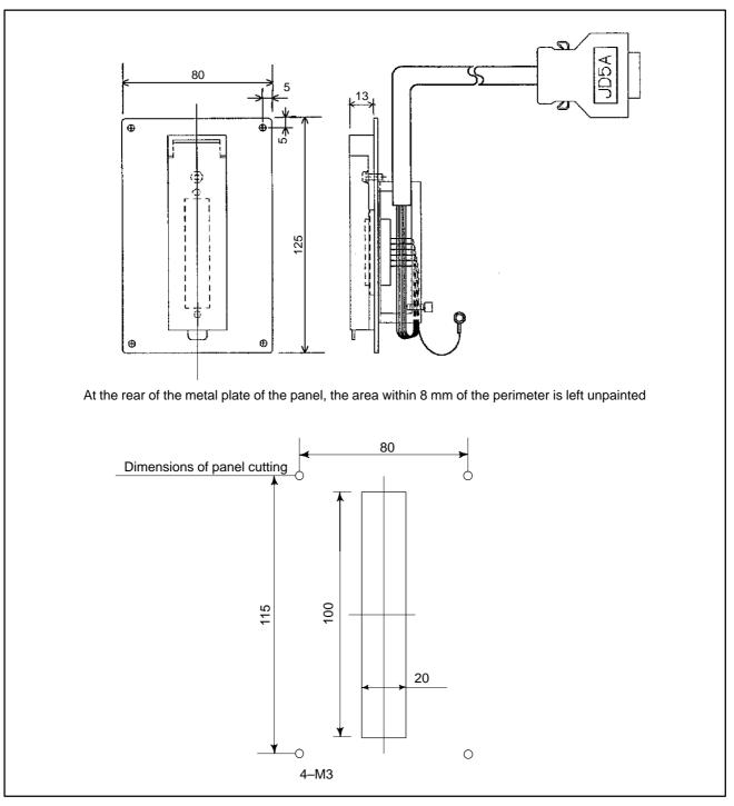
Fig.U23 Punch panel (wide width type) Specification No. : A02B–0120–C181 (Cable length : 1m) A02B–0120–C182 (Cable length : 2m) A02B–0120–C183 (Cable length : 5m)
