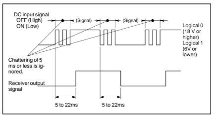
Fig. 9.9.1 (b) Signal width and delay of input signal
