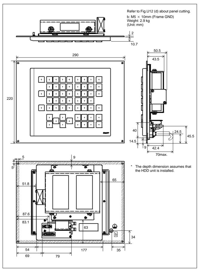
Fig.U11 (a) Stand-alone type standard MDI unit for CNC display unit with PC functions (10.4" LCD, vertical type)
