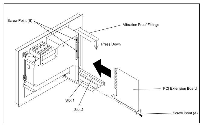
(3) Method of mounting PCI extension board
