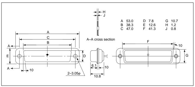
Fig.C8 (a) Punch panel connector for reader/puncher interface
