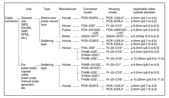
Fig. B.3 Cable connectors
