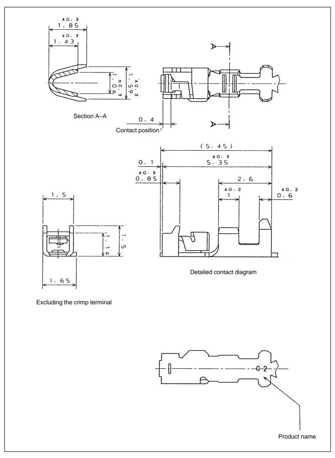
Fig.C7 (b) Contact (Japan Aviation Electronics)(for MDI)
