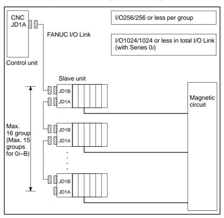
Fig.9.2 I/O Link connection diagram
