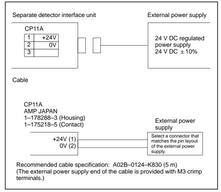
The 24 V DC input to CP11A can be output at CP11B for use in branching. The connection of CP11B is identical to that of CP11A. In this case, the power supplied to CP11A should be equal to the sum of the rating of the separate detector interface unit and that of the units after CP11B.
