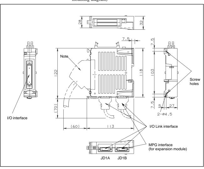
When mounting a module using screws (external module view and mounting diagram)
