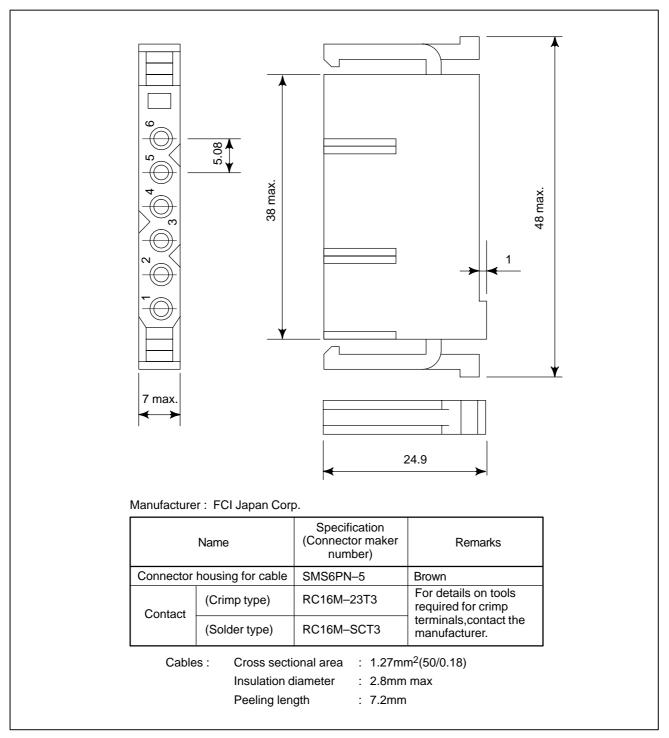
Fig.C5 Connector made by FCI Japan (6 pins,brown)
