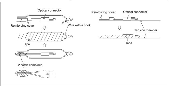
pull it. Because the combined tensile strength of the two cords is only 14 kg, however, avoid applying too great a force to the cable during installation, regardless of whether you have taken the protective measures.
