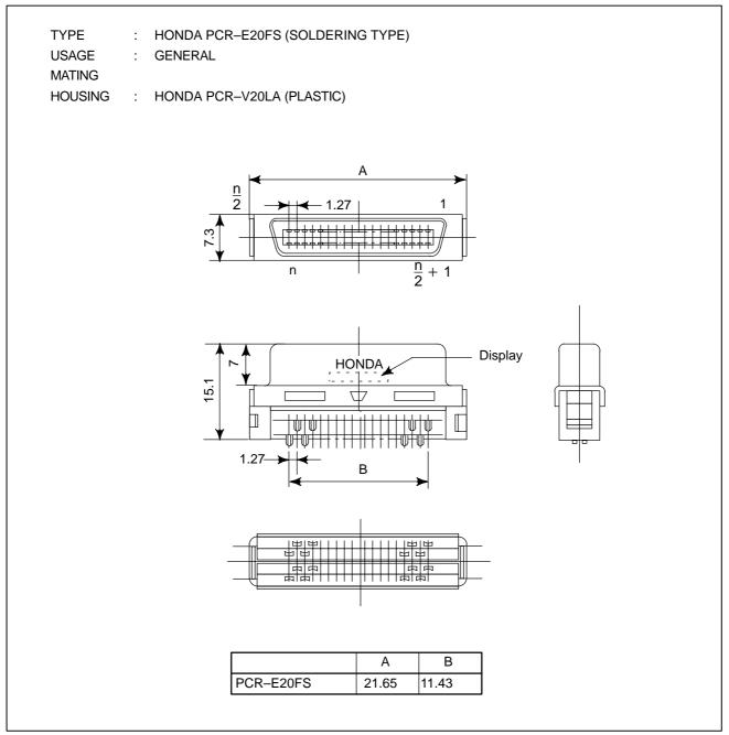
Fig.C1 (a) PCR connector (soldering type)
