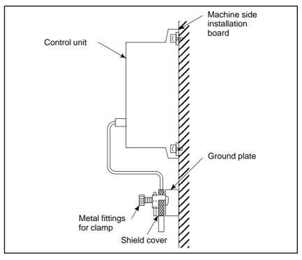
Fig.3.5.5(b) Cable clamp (2)
