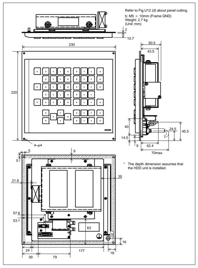
Fig.U11 (b) Stand-alone type standard MDI unit for CNC display unit with PC functions (10.4" LCD, horizontal type)
